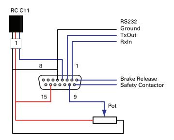
FIGURE 7. Factory Default Pins Assignment
