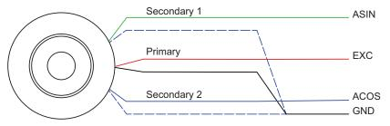
FIGURE 4. Resolver wiring
