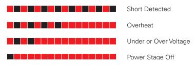
FIGURE 9. Exception or Fault Flashing Patterns
