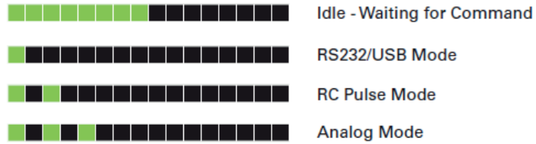
FIGURE 9. Normal Operation Flashing Patterns
