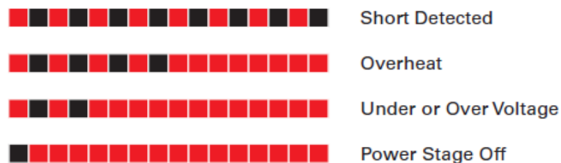
FIGURE 8. Exception or Fault Flashing Patterns
