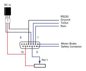
FIGURE 6. Factory Default Pins Assignment
