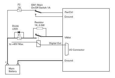
FIGURE 4. Contactor Wiring Diagram
