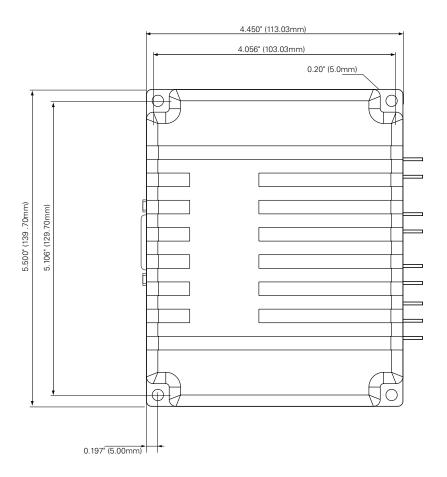
FIGURE 8. MDC1xxx Top View and Dimensions
