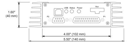
FIGURE 12. HDC24xx Front View and Dimensions
