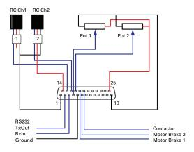
FIGURE 8. Factory Default Pin Assignment
