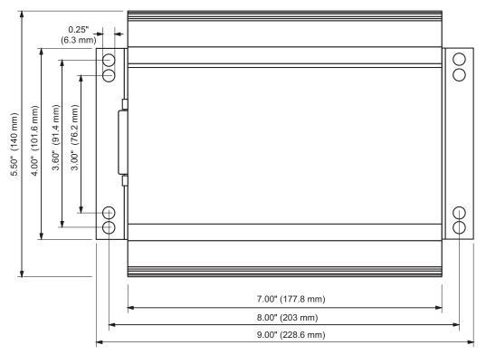
FIGURE 13. HDC24xx Top View and Dimensions
