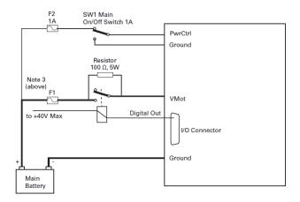
FIGURE 4. Contactor Wiring Diagram
