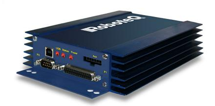
Roboteq's HDC2400 series controllers are designed to convert commands received from a RC radio, Analog Joystick, wireless modem, PC (via RS232 or USB) or microcomputer into high voltage and high current output for driving one or two DC motors. Designed for maximal ease-of-use, it is delivered with all necessary cables and hardware and is ready to use in minutes. Using CAN bus, up to 127 controllers can be networked at up to 1Mbit/s on a single twisted pair.
