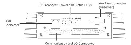
FIGURE 5. Front Controller Layout
