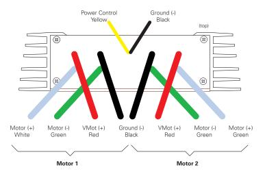
FIGURE 1. Rear Controller Layout
