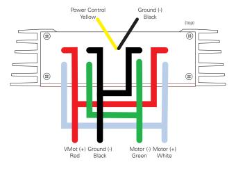
FIGURE 3. Controller wiring for single channel operation
