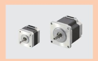
This is a high torque and low vibration stepper motor with a basic step angle of 0.72° (resolution of 500 steps per revolution).
