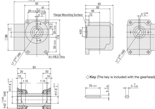
Cross Section AA (Detail Drawing of Output Shaft)
