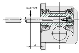
Lp (mm): Distance from flange mounting surface to overhung load point
