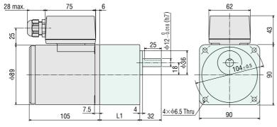
(The key is included with the gearhead)  $25_{\pm 0.2}$  3  $4_{-0.03}^{0}$   $4_{-0.03}^{+0.040}$  3  $4_{-0.040}^{+0.040}$  3
