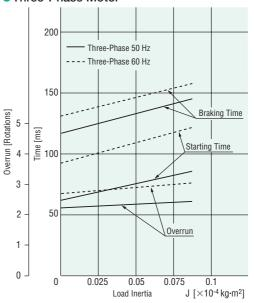
Electromagnetic Brake Motors
