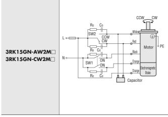
SW1 operates both motor and electromagnetic brake action. The motor will rotate when SW1 is switched simultaneously to ON. When SW1 is switched simultaneously to OFF, the motor stops immediately with the electromagnetic brake and holds the load.
