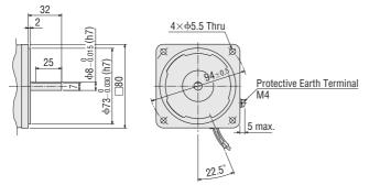
♦ Decimal Gearhead Can be connected to GN pinion shaft type. 4GN10XS Mass: 0.4 kg
