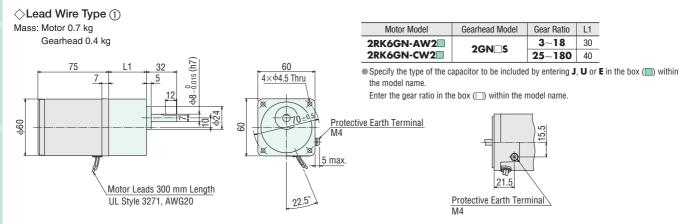
Detail Drawing of Protective Earth Terminal
