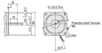
$\Diamond$ Decimal Gearhead Can be connected to **4TK10GN** type. 4GN10XS Mass: 0.4 kg
