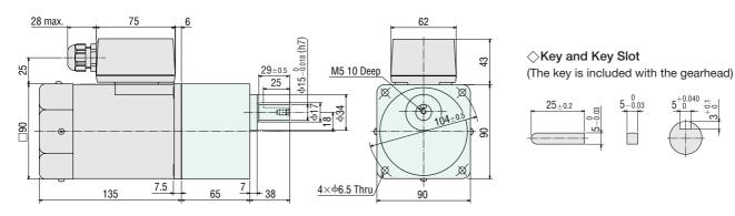
• Use cable with a diameter of  $\phi 6 \sim \phi 12$  mm.
