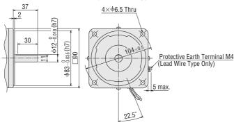
Oecimal Gearhead Can be connected to GE pinion shaft type. 5GE10XS Mass: 0.6 kg
