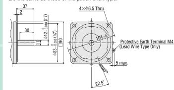
♦ Decimal Gearhead Can be connected to GE pinion shaft type. 5GE10XS Mass: 0.6 kg
