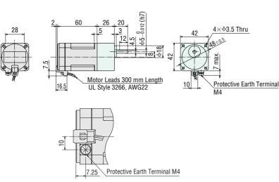
Detail Drawing of Protective Earth Terminal
