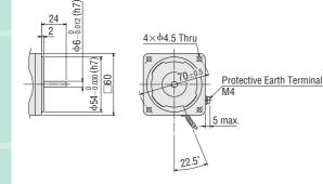
◇Decimal Gearhead Can be connected to GN pinion shaft type. 2GN10XS Mass: 0.2 kg
