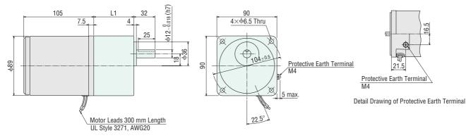
◇Terminal Box Type ② Mass: Motor 2.6 kg Gearhead 1.5 kg
