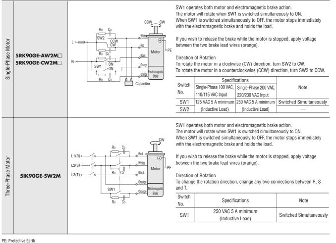
$\bullet$  R<sub>0</sub> and C<sub>0</sub> indicate surge suppressor circuit. [R<sub>0</sub>=5~200  $\Omega$ , C<sub>0</sub>=0.1~0.2  $\mu$ F, 200 WV (400 WV) ] EPCR1201-2 is available as an optional surge suppressor. → Page 123
