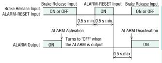
It is also possible to deactivate the alarm by turning off the power and turning it on again. Turn off the DC or AC power, and turn all input signals "OFF" before turning on the power again.
