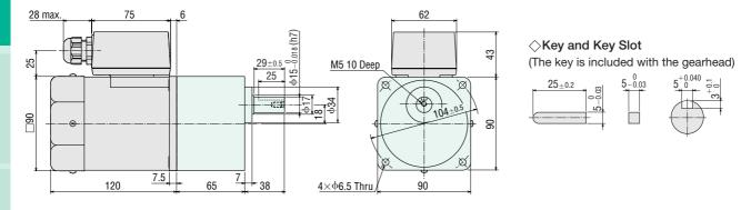
• Use cable with a diameter of  $\phi 6 \sim \phi 12$  mm.
