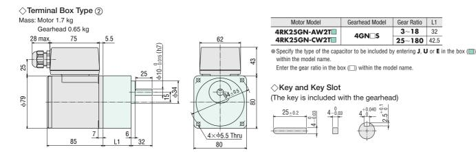
$\bullet$  Use cable with a diameter of  $\varphi 6 \sim \varphi 12$  mm.
