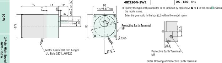
Detail Drawing of Protective Earth Terminal
